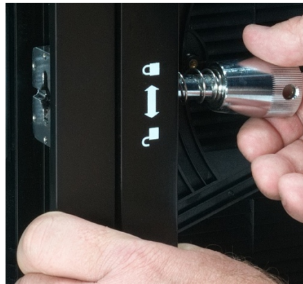
1. Align the locking-tab with tab-keyed connector socket
